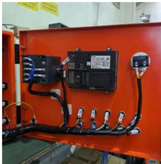
Gambar 2. 2 Wrapping spiral kabel Pokayoke Tightening Device
