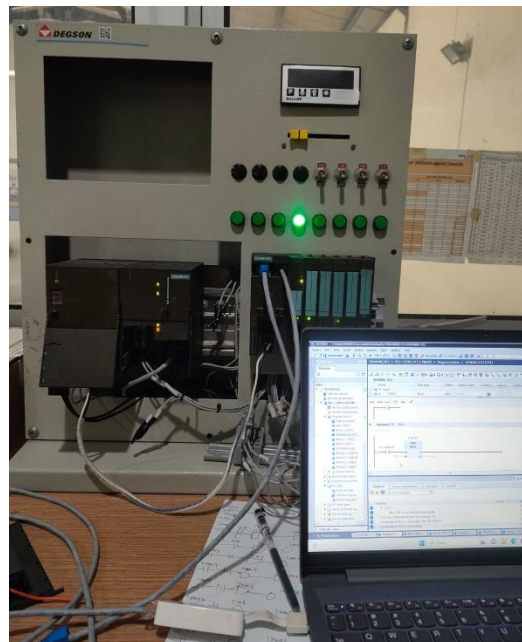
Gambar 2. 2 Training PLC SIEMENS
