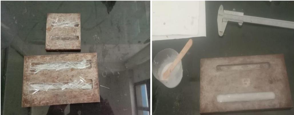
Gambar 3. Proses pencetakan sample
