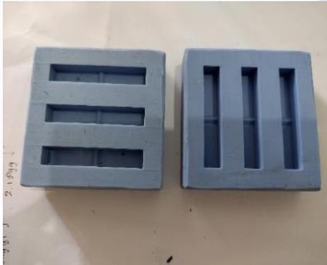
Gambar 3.5 Cetakan Spesimen Standar ASTM E23
