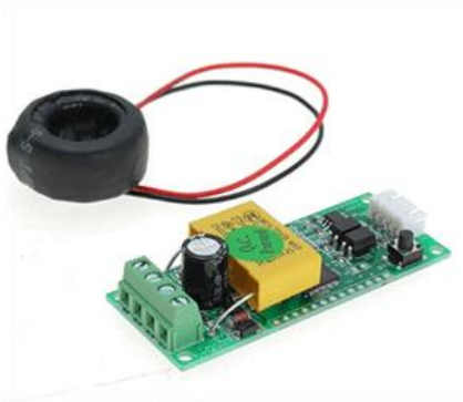
Gambar 2. 10 Sensor Arus PZEM-004T [12]
