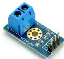
Gambar 2. 12 Sensor Tegangan DC [14]
