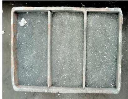
Gambar 3.6 Kotak Carburizing.
