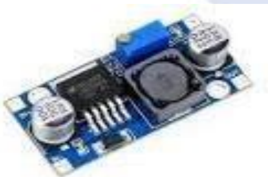
Gambar 2.4 DC STEP DOWN
