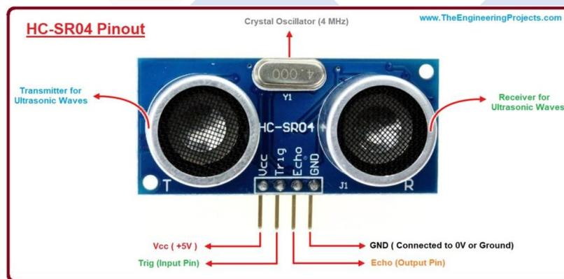
Gambar 2. 5 Sensor Ultrasonik [12].
