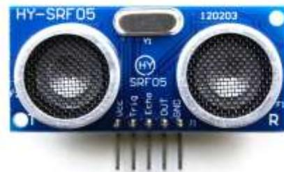
Gambar 2. 6 Sensor Ultrasonik HY-SRF05
