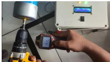
Gambar 4.5 Pengujian C Infrared Speed Sensor LM 393
