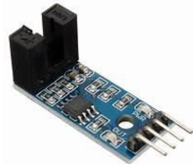
Gambar 2.4 Infrared speed sensor LM 393
