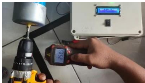
Gambar 4.3 Pengujian A Infrared Speed Sensor LM 393
