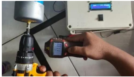
Gambar 4.4 Pengujian B Infrared Speed Sensor LM 393
