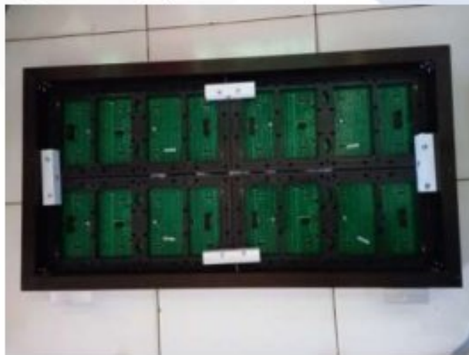
Gambar 4.2 Perakitan Display Led Dot Matriks Tampak Belakang
