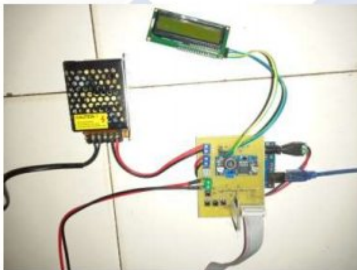
Gambar 4.6 Pemasangan unit power supply
