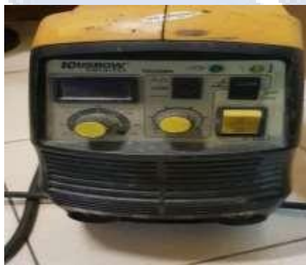
Gambar 3.4 Mesin Las SMAW KRISBOW kw14-722 Inverter TIG Welding 200A
