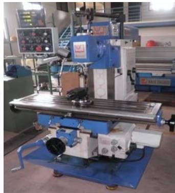
Gambar 2. 4 Mesin Frais Universal Knuth UFM 2 [12]
