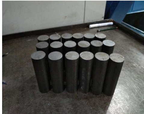
Gambar 3. 8 Baja AISI 1045 diameter 30 mm
