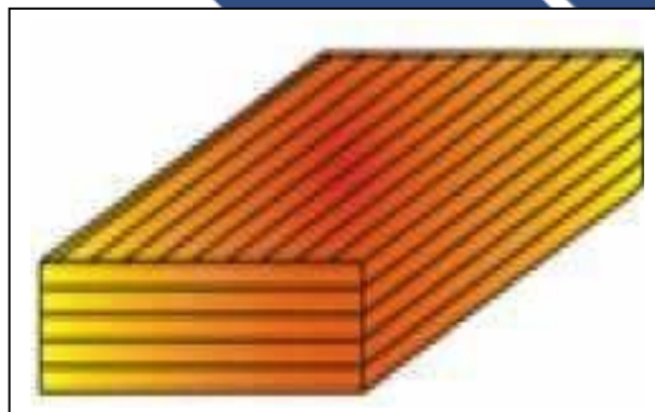
Gambar 2.3 Continuous fiber composite (Widiarta, 2018)
