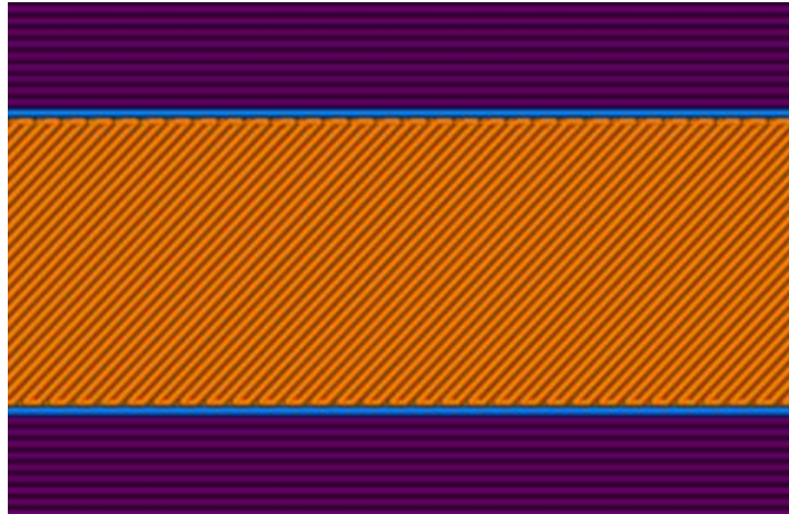
Gambar 2. 4 Infill Pattern Rectilinear
