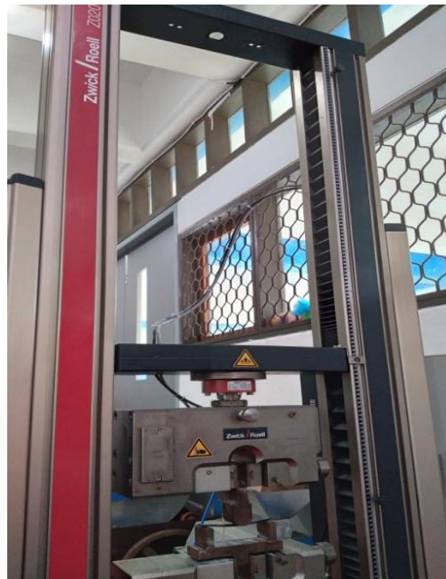
Gambar 3.4 Mesin Pengujian Bending Zwick Roell Z020
