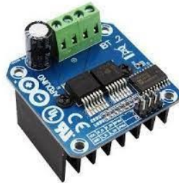
Gambar 2.9 Driver Motor IBT-2 [14]
