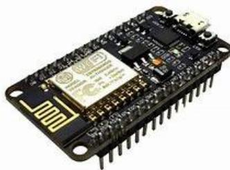
Gambar 2. 2 NodeMCU ESP32
