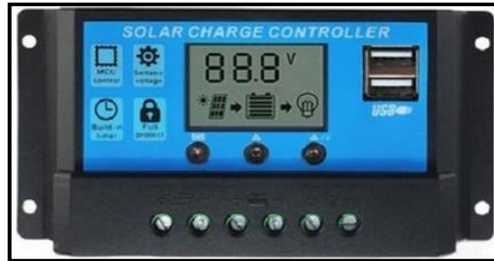
Gambar 2.20 Solar charger controller (SCC)
