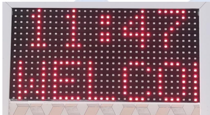
Gambar 4. 3 Pemasangan Led Matrix
