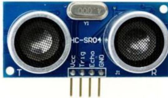
**Gambar 2. 3 Sensor Ultrasonik HC-SR04**
