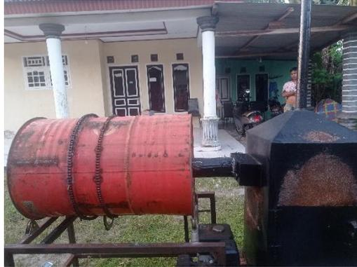
Gambar 3.5 Mesin *rotary dryer*
