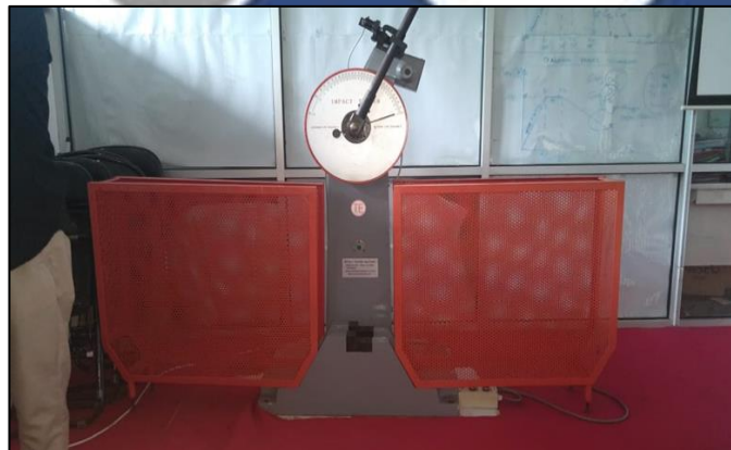
Gambar 4.8 Mesin uji impak Polman TESTING MACHINE metode Charpy model
