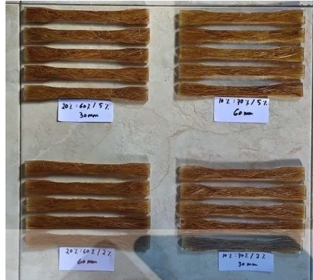
Gambar 4.8 Spesimen Uji Tarik (ASTM D-638)
