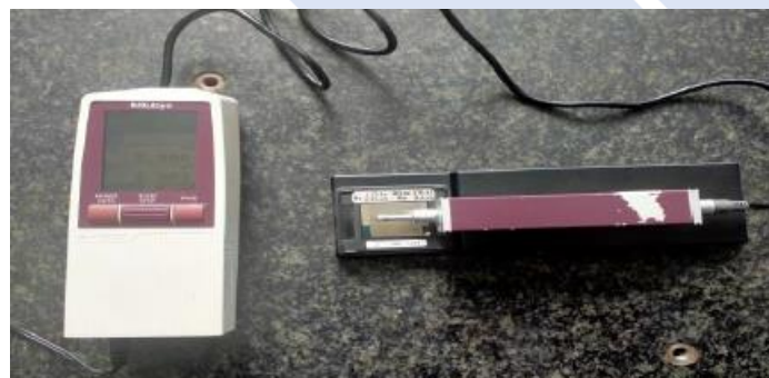
Gambar 3. 9 Pengkalibrasian alat uji surface roughness tester
