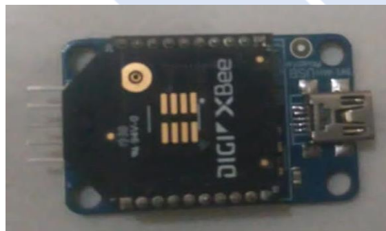
Gambar 3.3 Digi Xbee 3 PRO Zigbee 3.0 XB3-24Z8PT
