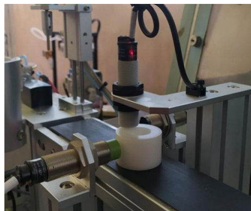
Gambar 4.11 Benda kerja melewati Sensor capasitive , sensor inductive , dan sensor photo
