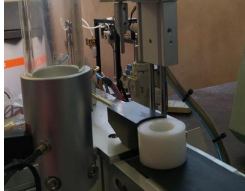
Gambar 4.10 Silinder move mendorong benda kerja ke conveyor
