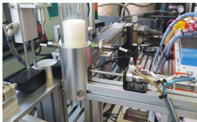
Gambar 4.20 Silinder supply mendorong benda kerja
