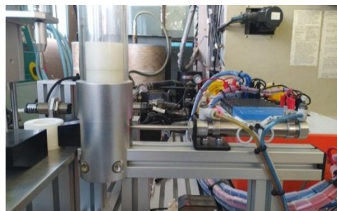
Gambar 4.9 Silinder supply mendorong benda kerja
