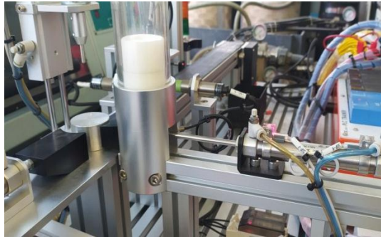
Gambar 4.14 Silinder supply mendorong benda kerja
