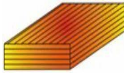
Gambar 2.6 Continuous Fiber Composites [12].
