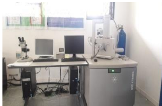
Gambar 3.9 Alat Uji Scanning Electron Microscope (SEM) Inspect S50
