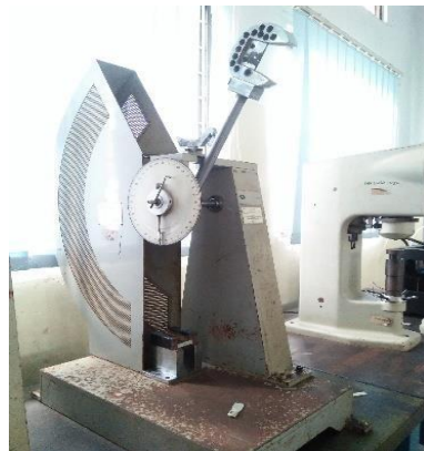
Gambar 3.14 Alat uji impak GOTECH Model GT-7045
