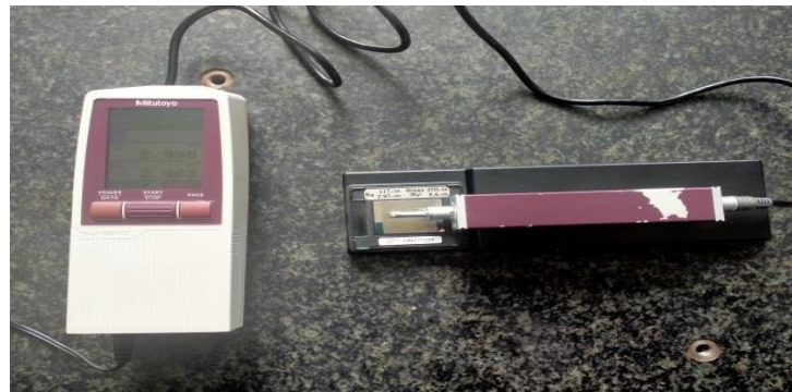
Gambar 3.9 Pengkalibrasian alat uji surface roughness tester
