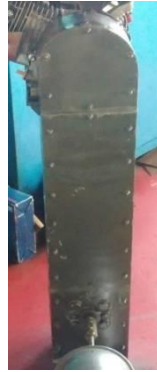
Gambar 4. 6 Pemasangan Cover Penutup Pulley Belt
