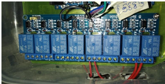
Gambar 4.5 Pengujian Modul Driver Relay 8 chanel .
