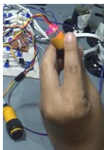
Gambar 4. 17 Pengujian sensor proximity infrared
