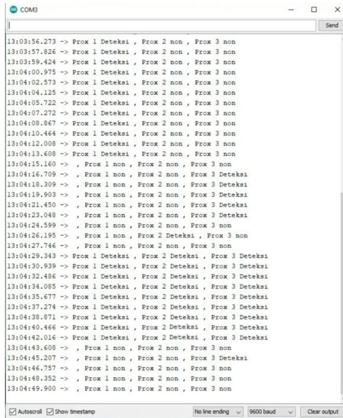
Gambar 4. 16 Serial monitor pengujian sensor proximity infrared
