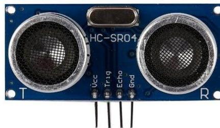
Gambar 2.4 Sensor *ultrasonic HC-SR04* [6]
