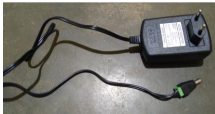
Gambar 4.4 Adaptor 5VDC 3A
