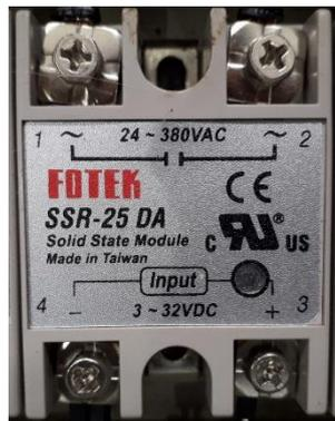
Gambar 2.10 *Solid State Relay*
