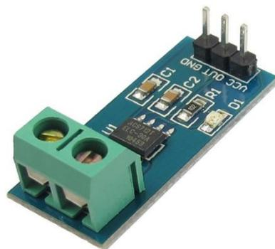
Gambar 2.8 Sensor Arus ACS 712 30A[12].
