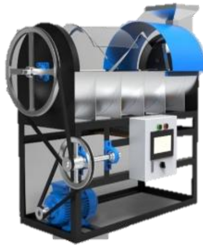
Gambar 2.5 Mesin sangrai kacang tanah berbasis programmable logic controller (PLC) dan supervisory control and data acquisition (SCADA) [9].
