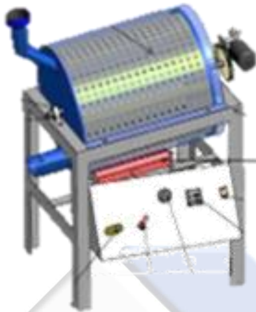
Gambar 2.6 Mesin sangrai kopi semi otomatis type drum rotary [10].
