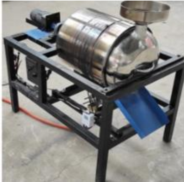
Gambar 2.3 Mesin sangrai kopi semi otomatis type drum rotary [11].
