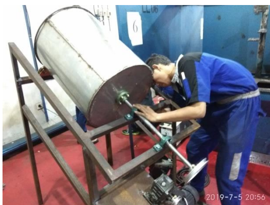
11. Assembly Tabung, Reducer dan Motor
