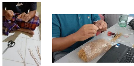
Gambar 9. Proses pelintiran serat sawit
