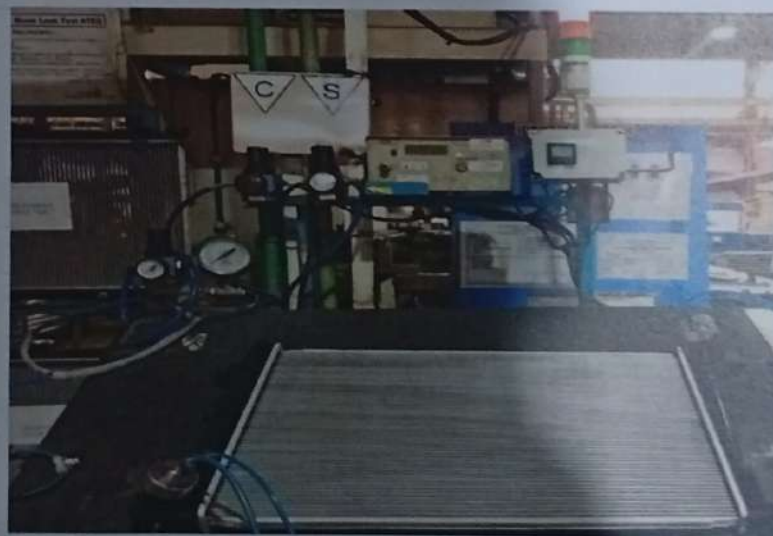
Gambar 1.13 Mesin Radiator Leak Test
