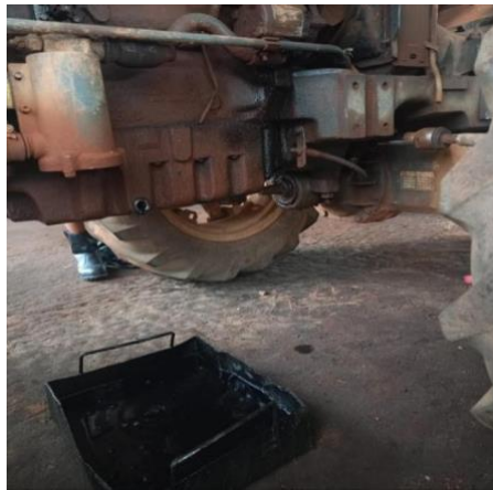
Gambar 2. 14 Ganti Oli, Filter Traktor Landini 8860
