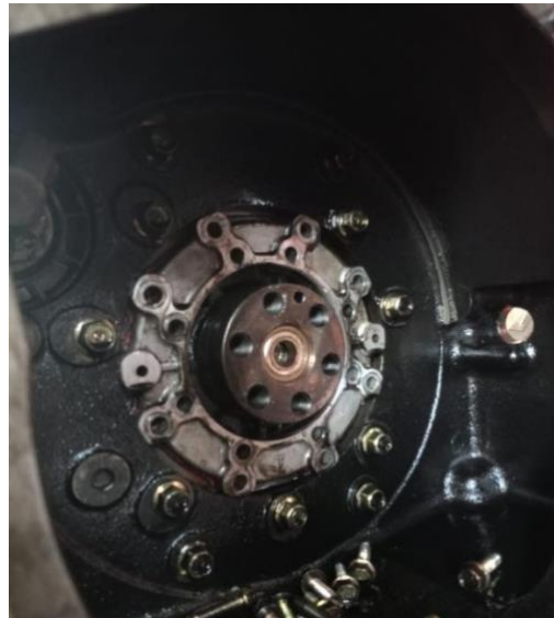
Gambar 2. 10 Ganti Seal Crankshaft Traktor Kioti 3503-D\
