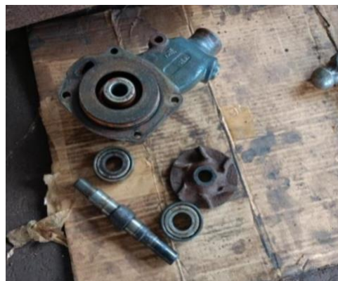
Gambar 2. 17 Perbaiki Water Pump Traktor Landini 8860
