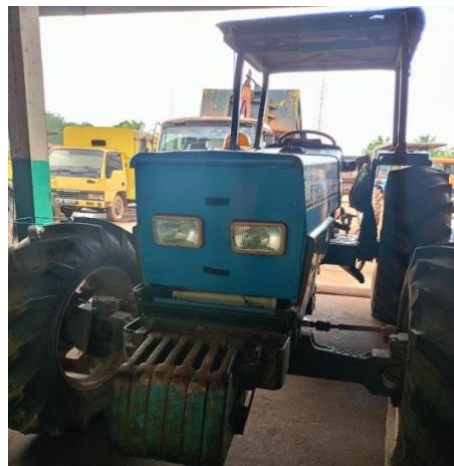
Gambar 2. 8 Pasang Lampu Traktor Landini 8860
