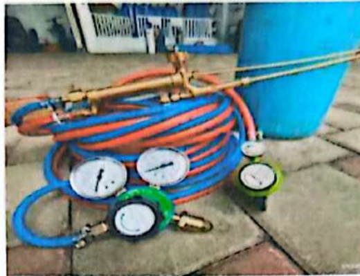
Gambar 9. Blender Las (Welding Torch)
