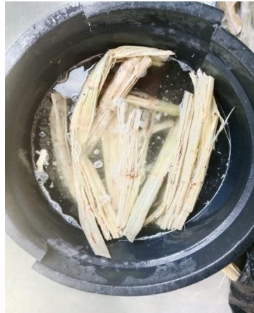
Gambar 3. 12 Proses Pencucian Ampas Tebu
