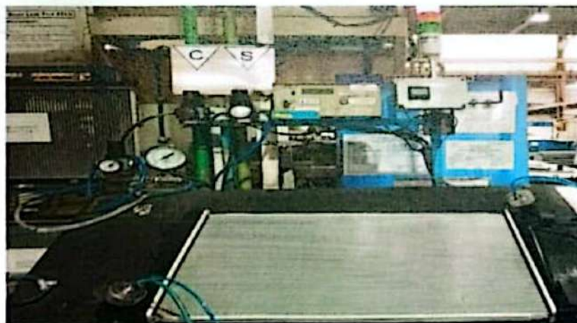
Gambar 1.14 Mesin Radiator Leak Test
