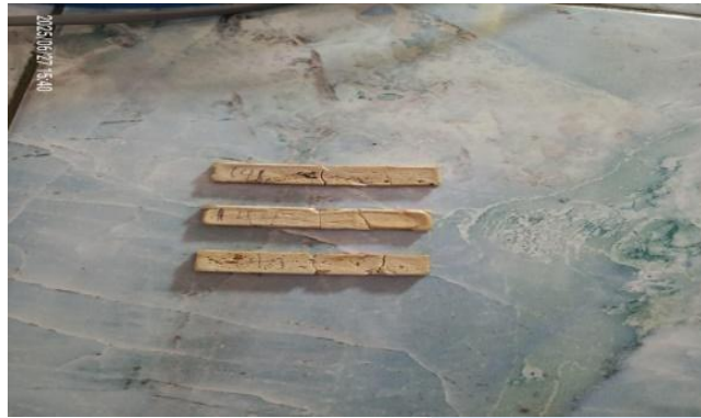
Gambar 4.6 Sampel uji impact 0,75gr talc resin
