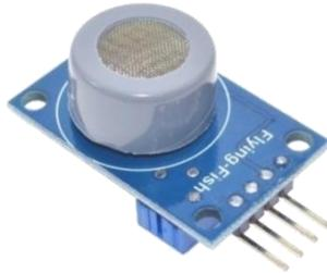
Gambar 2.4 Sensor MQ7 (*Pixel Electric Engineering, 2018*)
