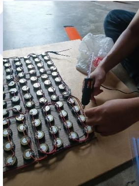
Gambar Lampiran 3. 12 Proses Penempelan Lem Lilin
