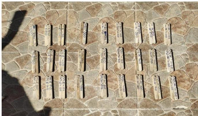
Gambar 4. 1 Spesimen Uji Tarik Dan Uji Bending.
