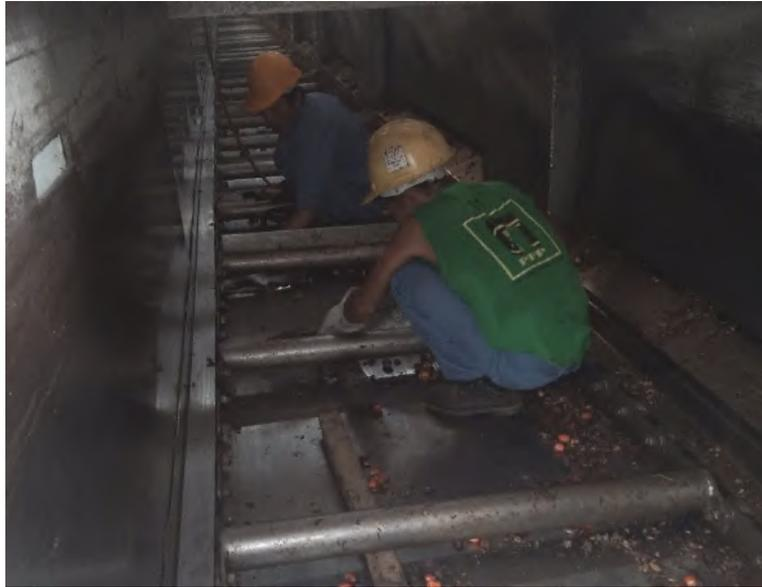
Gambar 2. 5 Pergantian *Liner/Rel Conveyor FFB*
