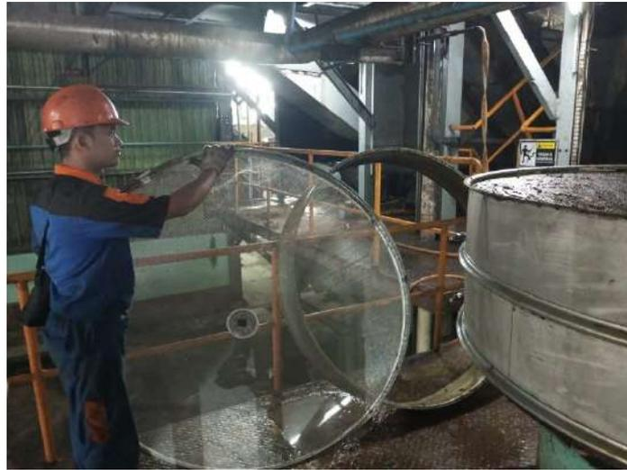
Gambar 2. 16 Pergantian Saringan *Vibrating Screen DCO*
