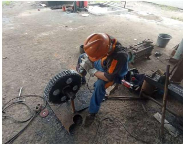
Gambar 2. 10 Merekon *Gear Band Crusher*
