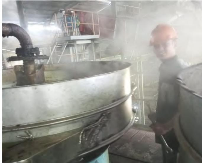
Gambar 2. 18 Pergantian Saringan *Vibrating Screen Sludge*
