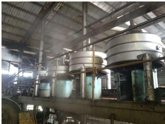
Gambar 2. 17 *Vibrating Screen Sludge*
