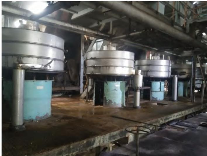
Gambar 2. 15 *Vibrating Screen DCO*
