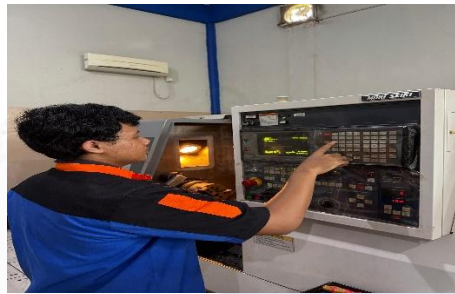
Gambar 3. 10 Proses Input Program CNC
