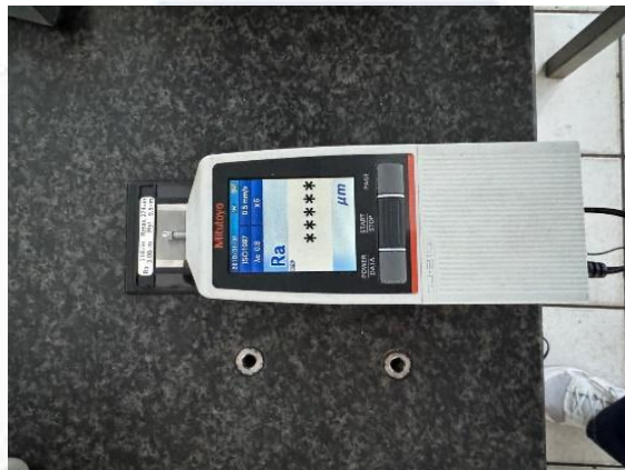
Gambar 3. 6 Surface Roughness Tester Mitutoyo SJ-210
